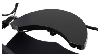
Four switch proximity array
