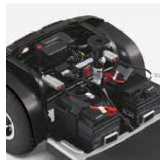
Built in anti-splash guards Protects electronics and the transaxle from dirt and water.
