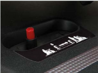
Two-step disengaging lever to prevent free-wheeling
