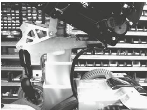
Lifter column completely extended.
