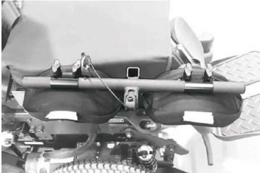
Fig. 6-1 Knee bolster assembly in stowed position
